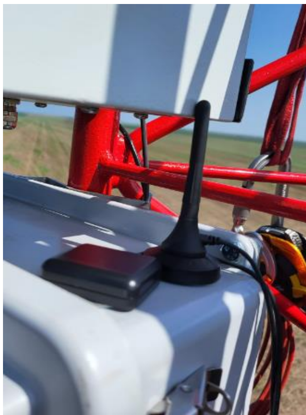
Pictures of antenna outside the logger cabinet
