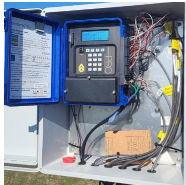
Picture from Logger cabinet inside
